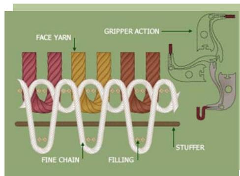
The precision of the weaving process, along with the intricate construction of an Axminster carpet, ensures the carpets strength and dimensional stability to support the design intent in severe traffic areas.
