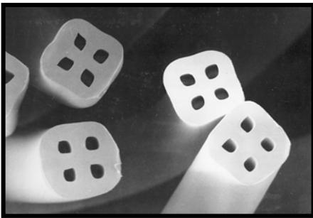
*Nylon Type 6.6 hollow core and round cross-sections*
