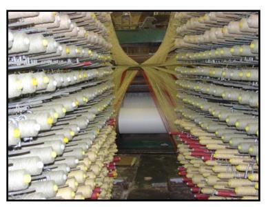
To create a 27" wide sample on a typical 216 pitch Wilton 3-frame loom would require the manufacturing, metering, and creeling of 648 unique yarn packages. The same sample on an 8 color gripper Axminster would require 1,512 unique yarn packages. While that was the typical sample method prior to the invention of the computer, technology has come to the rescue of making carpet samples.
