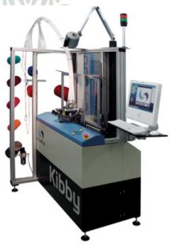
Utilizing a precision series of metal peg boards, the Kibby machine process cuts and positions individual points of yarn from a single yarn package, creating the desired patterns in the actual yarn dyed colors.
